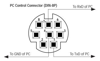
**NOTE:** Pins 2, 3, 5, 6 and 8 are used inside the projector.
